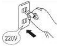
The outlet used for the machine's current must be greater than the machine's specified value; otherwise it may lead to overheating or fire.
