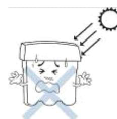
When the water purifier is in sunlight for a period of time, it may create a breeding ground for microorganisms so the water purifier water quality will decrease, and they may pollute the internal components of the water purifier.
