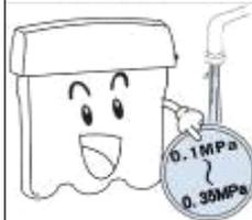
Operating under high pressure conditions may cause the water purifier pipes to rupture, resulting in leakage, the machine working improperly, or even serious property damage.
