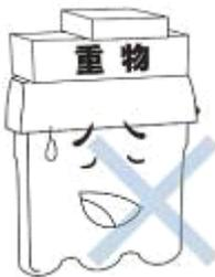
If heavy objects are placed on the water purifier, it may result in damage to the water purifier's dust cover or internal components, which could lead to leakage, the machine working improperly, or even serious
