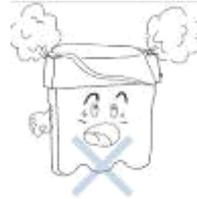
Obstructing the heat dissipation may lead to machine damage or fires.
